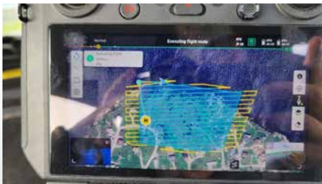
Figure 1: Photo of the flight line pathway over the old Rossville Cemetery. Bottom left of the screen shows the LiDAR point-clouds being collected.
